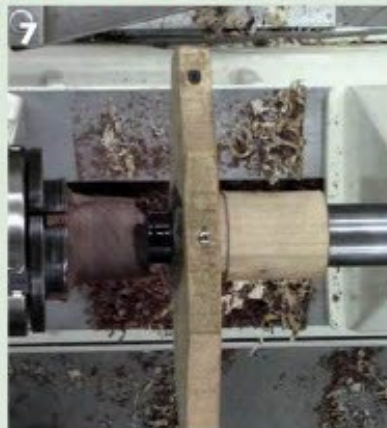
7 Cut a slight chamfer on the end of the spigot and use a die to cut threads on the spigot. You'll also need to undercut the last thread with a narrow parting tool.
