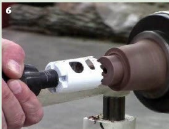
6 After bringing the bottom to round, use a hole saw to create a spigot on the end. Shape a perpendicular shoulder at the base of the spigot.
