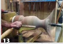
With a custom-turned, cone-shaped plug fit into the vase's opening and tailstock support in place, finish shaping the lower section of the vase's body.
