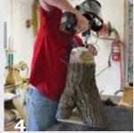
The piece is initially driven by a spur drive, allowing for adjustible positioning. Turn a flat base to accept a faceplate, the preferred and safer holding method for hollowing.
