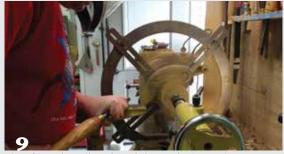
View from the tailstock end shows the intermittent cutting action—air and wood.
