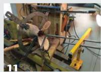
The author's captive boring bar setup. Hollowing only proceeds midway into the body at this stage. The vase's wings do not affect the actual hollowing process, other than adding the obvious danger of striking your hands or arms. Be ever mindful of the rotating wings.
