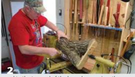
A wooden wing-support piece screwed to the top end of the branches receives the tailstock live center and allows for intentional positioning of the turning axis.
