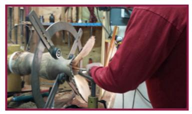
**21.** Turning the tendon on the base for holding onto it for final sanding.
