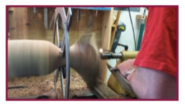
**12.** Starting from the outside, a push or pull cut can be made to round and shape the neck of the vase. The cut should be stopped short of the top edge so that the bark is not torn off. Make a push cut from
