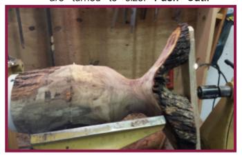
**9.** Steady rest is mounted and start shaping the top side of the wings of the crotch.
