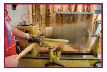
**6.** Rounding up the middle of the vase and shaping the underside of the wings of the crotch..
