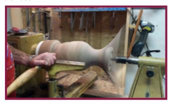
**18.** Put the steady rest back in place and set up the Hollowing system again to hollow out the bottom half of the vase. You can see the laser on this picture.
